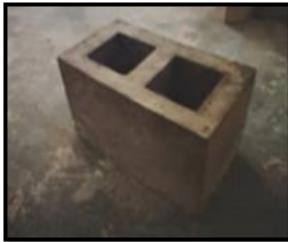
Figure 5: Concrete Hollow Block (320mm(L)x180mm(H)x180mm(W))
