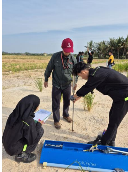
Figure 1: Mackintosh Probe testing at construction site
